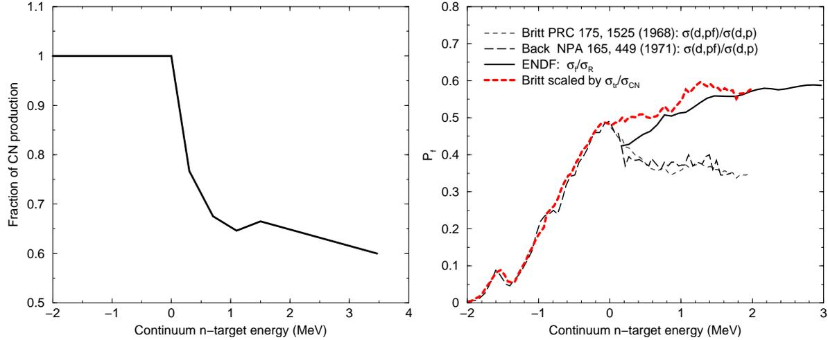
**Figure 3.** Results for the reaction  $d + {}^{239}\text{Pu} \rightarrow p + {}^{240}\text{Pu}$  at  $E_d = 15$  MeV. The left plot shows the probability of CN formation, as a function of energy across the neutron escape threshold. The right plot shows fission probabilities for neutrons incident on  ${}^{239}\text{Pu}$ : the new red curve shows the Brittr data divided by the CN formation probability of the left plot.
