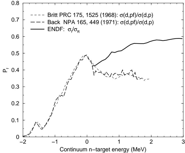
**Figure 1.** Fission probabilities for neutrons incident on  $^{239}\text{Pu}$ . Comparison of two surrogate experiments with probability from the ENDF/B.VII evaluation (the ratio of the fission cross section to the reaction cross section). The energy scale is  $E_n$ : the continuum neutron energy in  $^{240}\text{Pu}^*$ .
